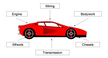
Figure 1 Major components of a vehicle.
